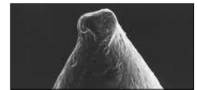
Typical swage-ballistic point finish results in potential failure of pin
