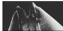
Typical cut-point finish resulting from manufacturing process will increase pin failure
