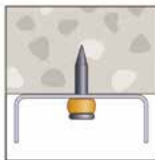
Setting aggregate is the biggest reason for overhead pin failure.
