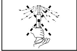
6. Never fire into very hard or brittle materials such as cast iron, tile, glass or rock. These materials can shatter, causing sharp fragments and/or the fastener to fly freely.
